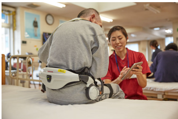
Fig. 3. Honda Assist ® (Rehab staff explaining data measured with controller wirelessly connected with Honda Assist ®)
