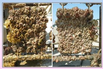
Status of Unpainted Test Plates When 12 Months Have Passed After Installment
